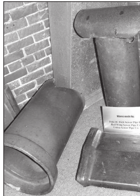
Sewer pipe tile was made from grittier, grainier clay. It was used to create Red Wing's infrastructure. Samples can be found in the Red Wing Pottery Museum.
