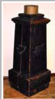
Right: A foundry pattern used to manufacture the base for the cast iron street lamp poles made for the City of Red Wing. Photos courtesy of Gary & Bonnie Tefft
